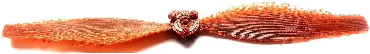
Fig. 15. Prototype of 3D printed propeller
