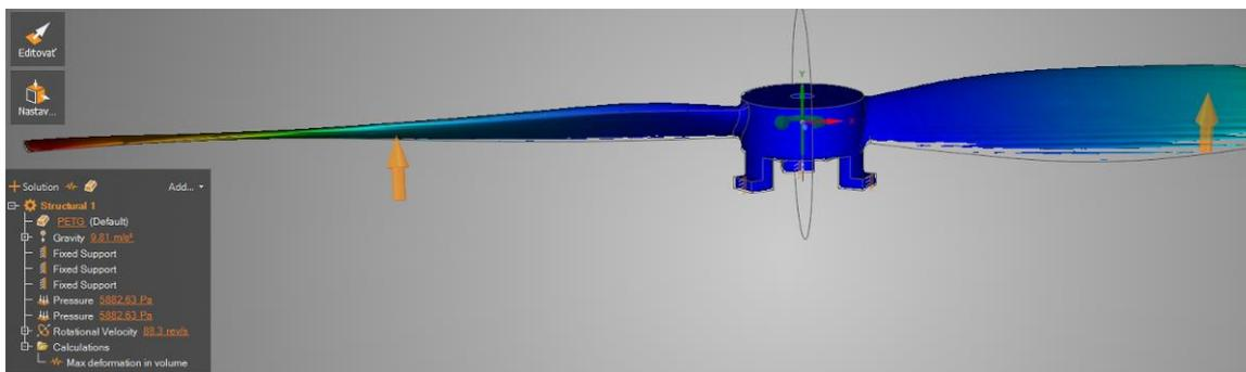
Fig. 6. Deformation of the propeller blade
