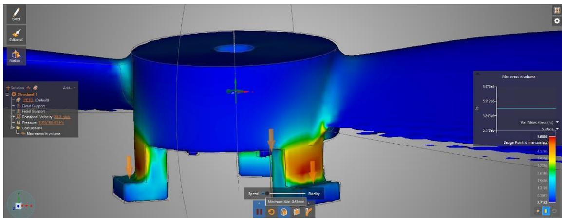
Fig. 9. Maximum stress in propeller legs for PETG
